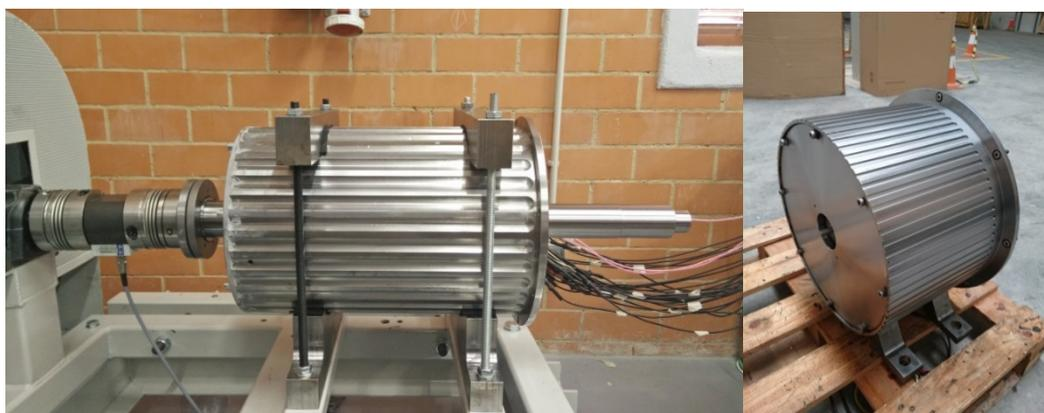
**Figure 1. H4 generator prototype (left) and H20 generator prototype (right)**
