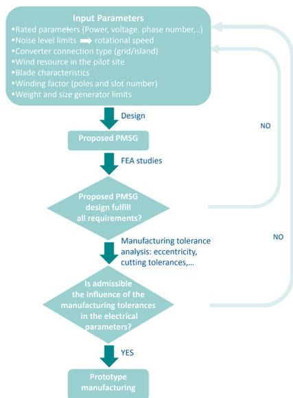
Fig. 1 Flowchart of PMSG design process.
