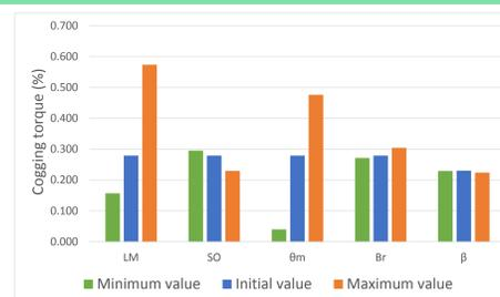
Fig.4 Manufacturing tolerance influence in Cogging torque (%).
