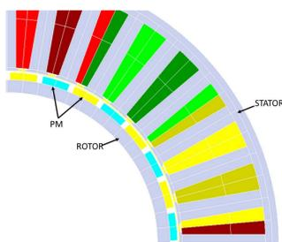
Fig. 2 2D Finite element model PMSG.
